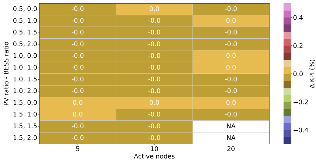
Fig. 3.12 Self-consumption rate (SC) variation with increasing numbers of active nodes, compared to the single active node case. Median values are displayed as a heatmap and shown numerically along with the range of variation in brackets (where applicable).
