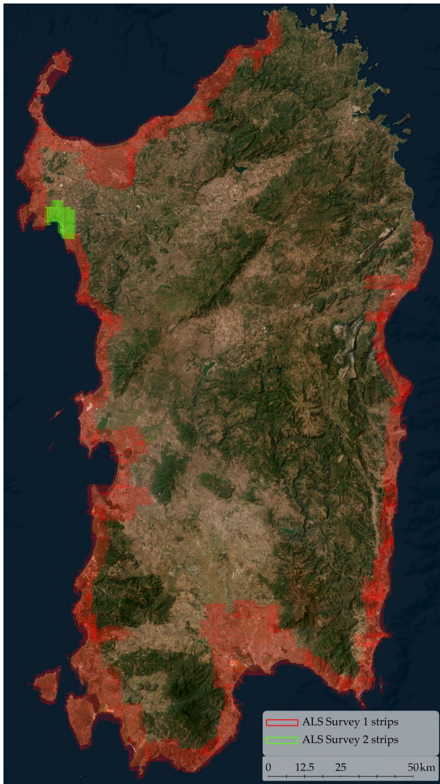
Figure 33. Map of the data provided by the Sardinia Region. The stripes available from the two airborne LiDAR surveys are located on this map. The two surveys were carried out using two different sensors, as detailed in Table 2. Datum WGS 1984, projection UTM zone 32 N (EPSG: 32632) – credits Sardinia region (data); author (elaboration).
