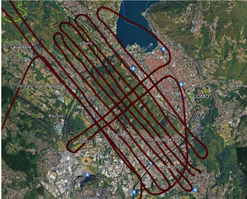
Figure 27. Flight pattern over the Spina Verde Park Case Study – credits CNR IRPI (data); CNR IRPI (Cappellazzo et. al, 2023) (elaboration).
