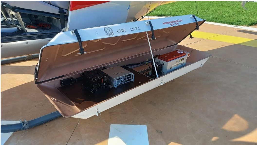
Figure 26. (a) Picture of the Eurocopter/Airbus AS350 used for the survey and (b) LiDAR pod containing the Litemapper LiDAR system, the GNSS/IMU platforms and the full frame PhaseOne camera – credits CNR IRPI.
