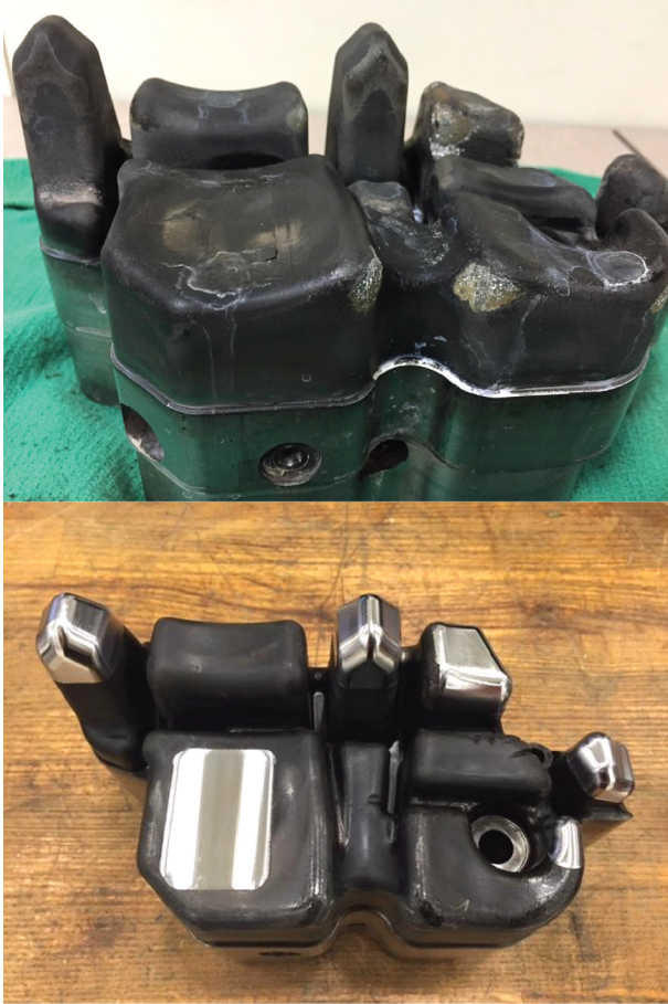
Fig. 1.1 Worn automotive die before and after the repair by DED-LB/Powder [7].
