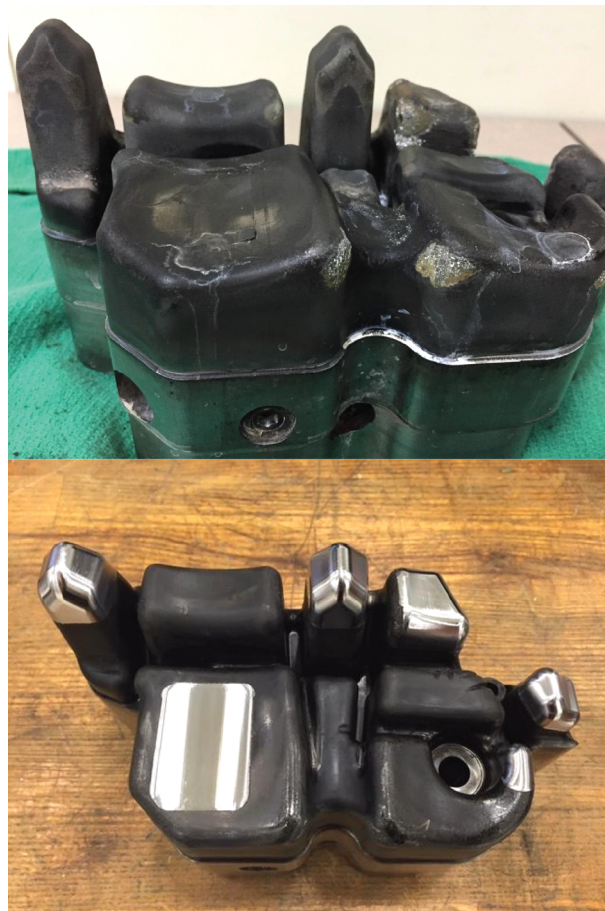
Fig. 1.2 Worn automotive die before and after the repair by DED-LB/Powder [34].
