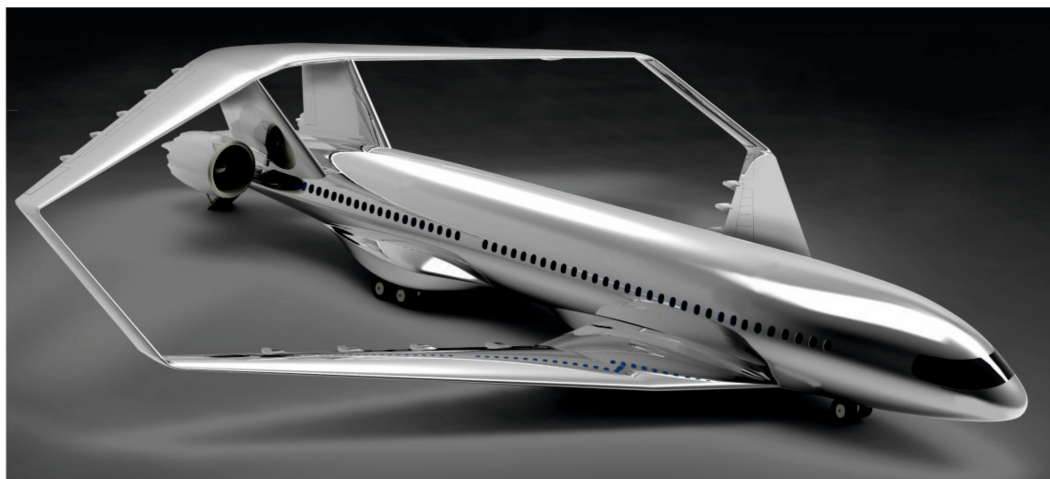
Figure 1. Representation of the PrandtlPlane (PrP) under development within the project “Prandtlplane ARchitecture for the Sustainable Improvement of Future AirPLanes” (PARSIFAL) [59].
