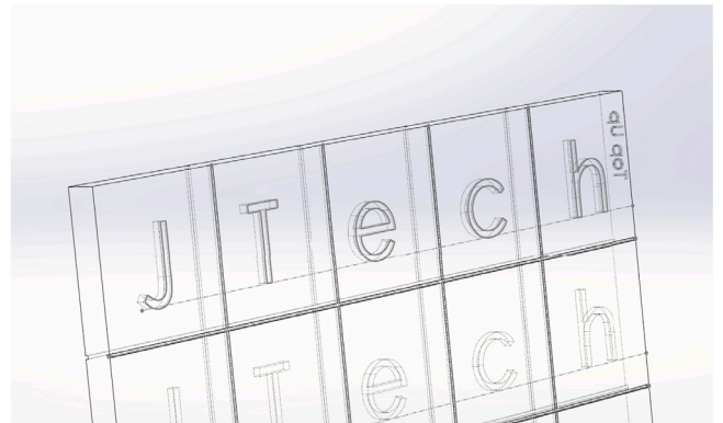
Fig. 11. Single plastic plate — overview of embedded characters composing the writing word “JTech”.
