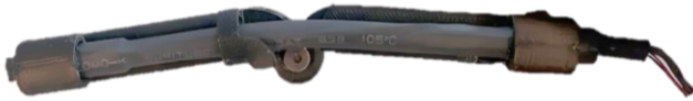
Fig. 2. 3D-printed testing rig used for characterizing the multimodal POF sensor's behavior during controlled F/E movements. The optical channel is securely positioned within the rig to ensure accurate testing conditions.
