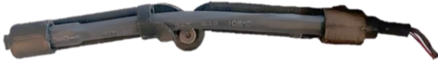
Fig. 2. 3D-printed testing rig used for characterizing the multimodal POF sensor's behavior during controlled F/E movements. The optical channel is securely positioned within the rig to ensure accurate testing conditions.
