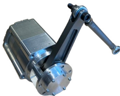
Figure 4. Electro-mechanical shock absorber prototype.
