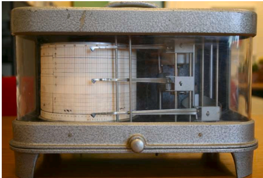
Fig. 2. Rainfall data recorder with paper roll adopted during the 20th century in many geographical areas of the World.
