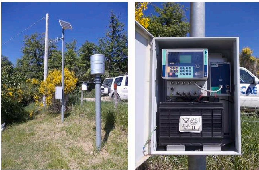
Fig. 3. Rain gauge station with tipping bucket sensor (left) and correspondent digital data-logger (right) installed in central Italy (Compresso, Umbria).
