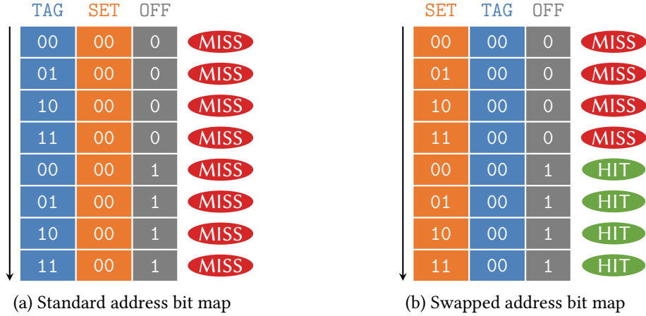
Figure 3.10: The sequence of B addresses accessed during the first 8 iterations of the matrix-matrix multiplication algorithm, where B \in \mathbb{Z}^{4 \times 8} has a 4-set direct-mapped cache. With the standard address bit mapping (a), the cache always misses since the same set is sequentially accessed by addresses with different tags, evicting the related line. Contrarily, the swapped address bit mapping (b) reads different sets with the same tag, achieving high hit rates.
