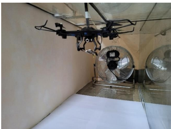
Figure 5 The drone in the wind tunnel.
