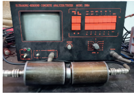
FIGURE 2: UTA2001A ultrasonic inspection monitor.
