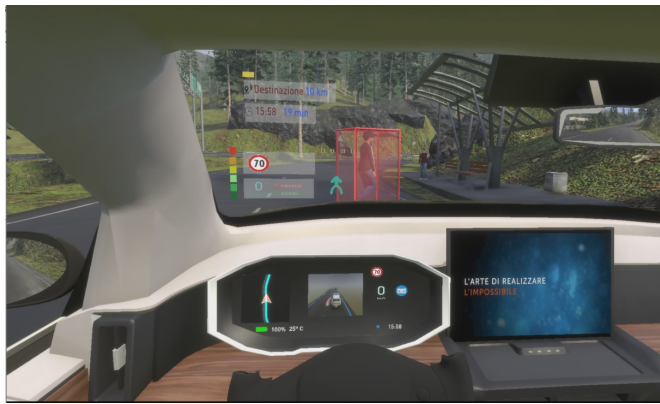
(c) 3D AR bounding box used to notify the jaywalker via visual cue
