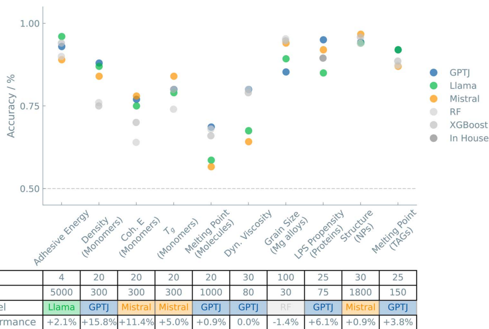
Fig. 1 Overview of the “Materials and properties” case studies. The accuracies of binary classifiers are plotted for the “Materials and properties” case studies. Three different LLMs (GPT-J, Llama, and Mistral) and two traditional ML models (random forest (RF) and XGBoost) are compared. The dashed line indicates the zero-rule baseline of 50% accuracy. The table summarizes the number of epochs (for fine-tuning the LLMs), training set size, the best-performing model, and the relative difference between the best LLM and the best “traditional” model.
