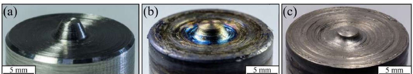
Figure 14. Butt FSW of 2.5 mm thick Ti6Al4V. (a) FSW tool produced from alloy ZhS6U before welding, (b) after \sim 2 m of welding, and (c) after \sim 2 m of welding without water cooling ( \omega 340–380 rpm, v 86 mm/min) [162].
