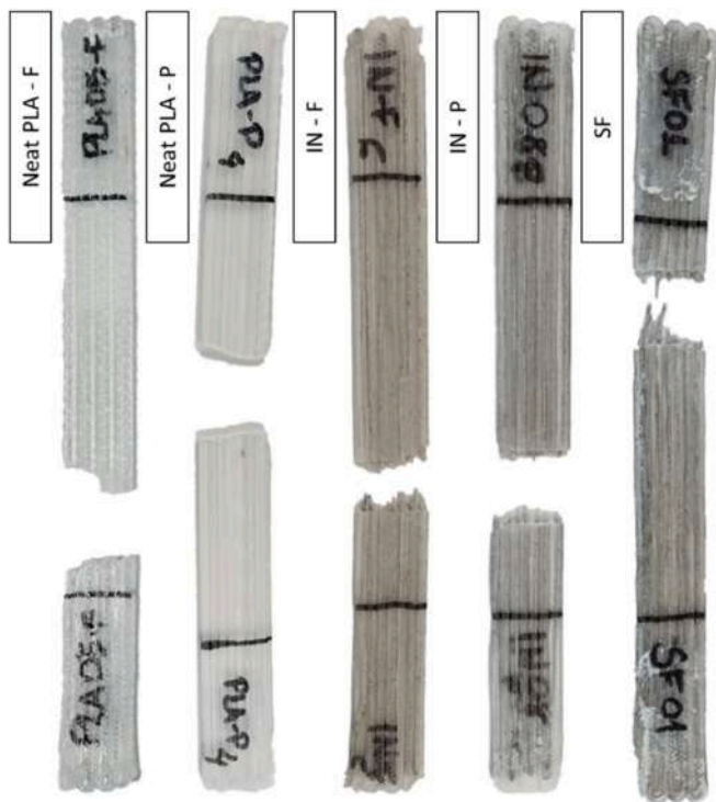
Fig. 17. Example of failure modes of the tensile samples.
