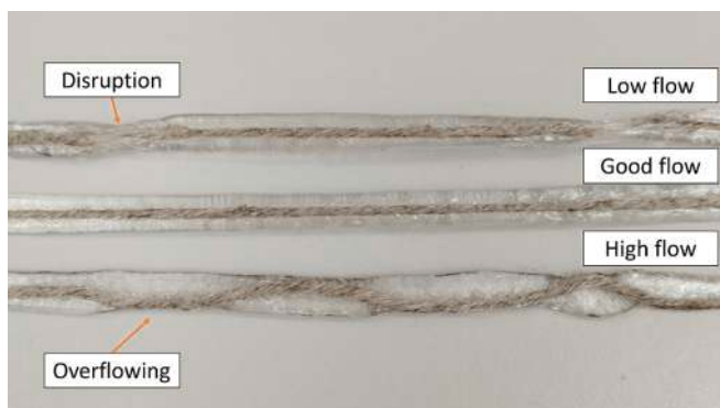
Fig. 11. Flow variation in the deposition rate test of flax composite filaments.
