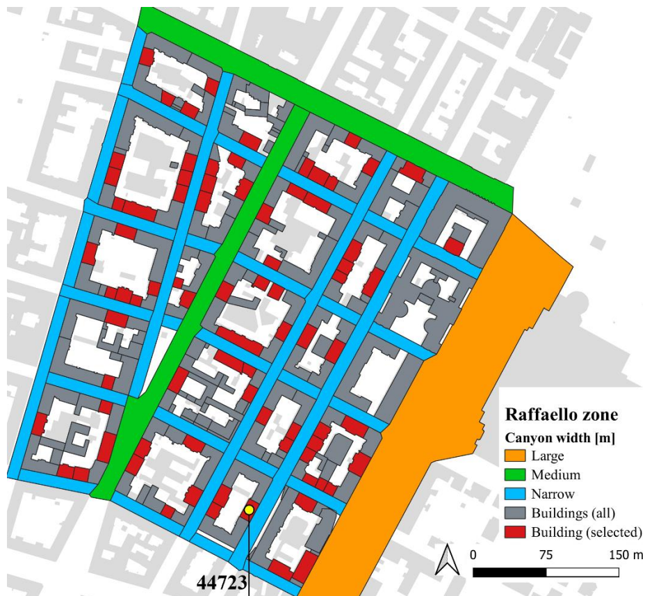
Fig. 90 – The examined building 44723 located in a narrow canyon Raffaello, NE-SW (30°N) oriented, and left positioned.
