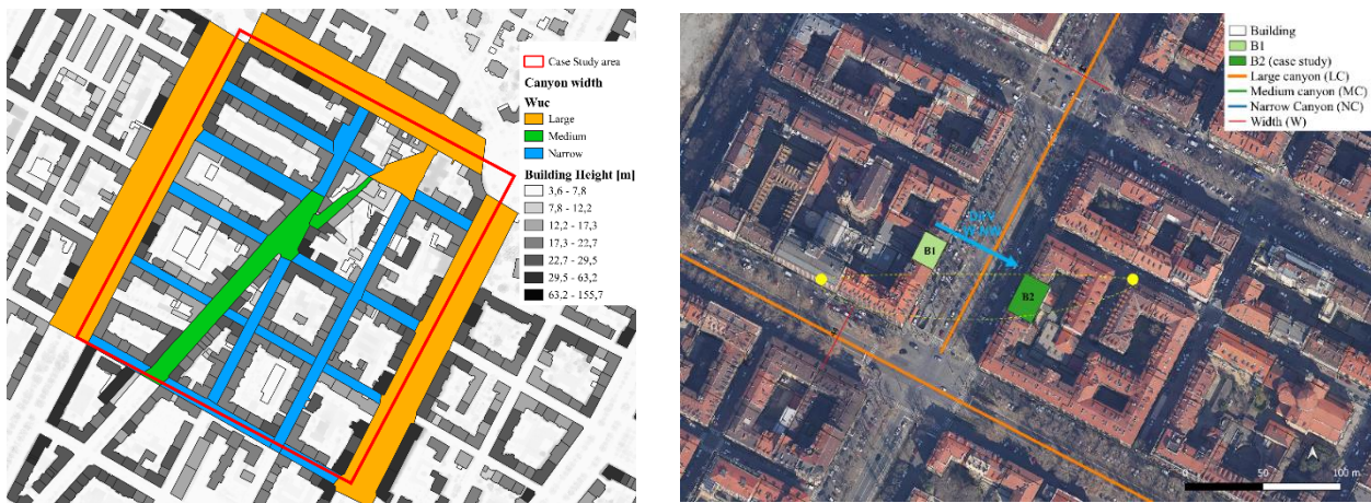
Fig. 50a-b - Localization of the urban canyons in Crocetta district for selected aspect ratios: narrow (blue), medium (green) and large (orange) (a), and the large urban canyon (LC) examined building with NE-SW axis, considering crosswind (DirV) and solar exposures (yellow dot) on the facades of building B1 and B2.
