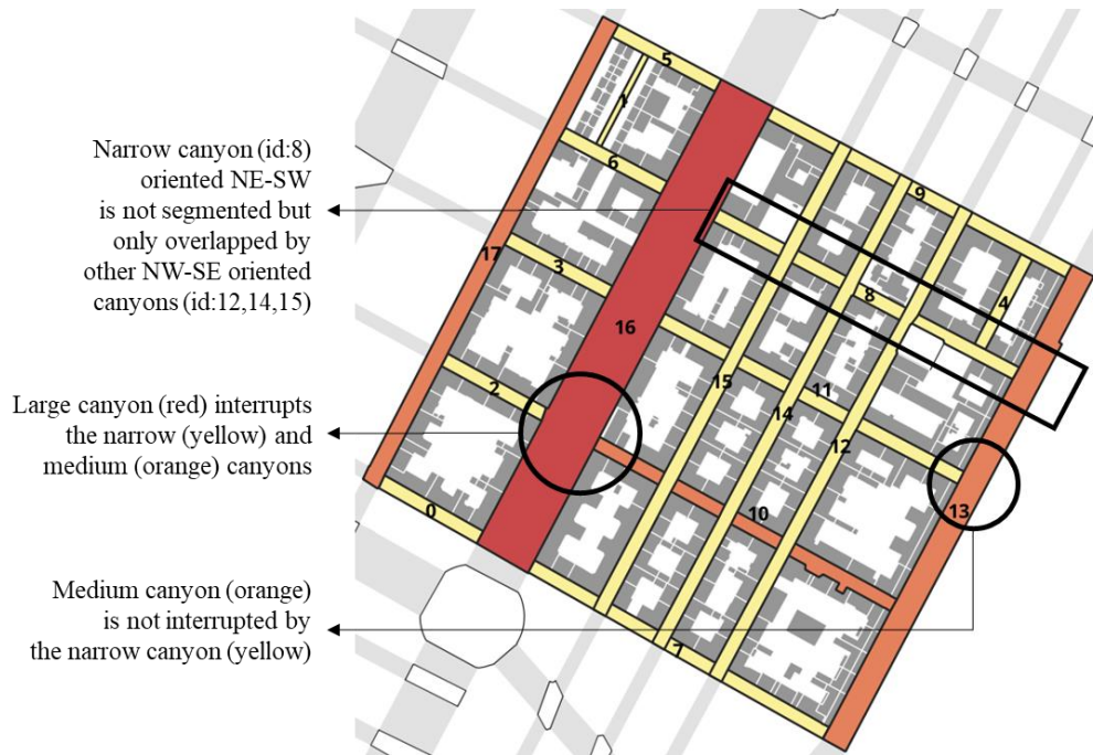
Fig. 45 - Example of the urban canyon layer in the geo-database with narrow (in yellow), medium (in orange) and large (in red) canyon width in a case-study zone in the city of Turin.
