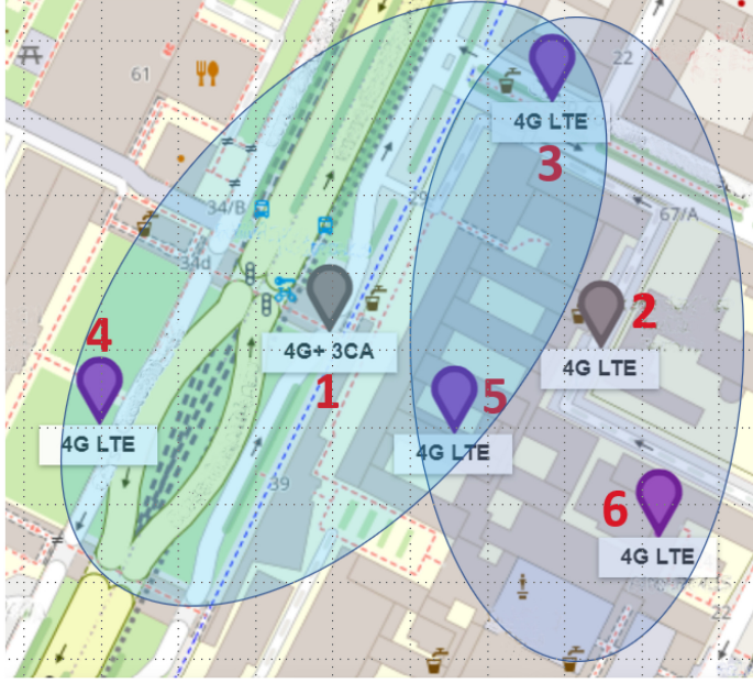
Fig. 6. Layout of the BSs covering a university campus. Macro cell BSs are in positions 1 and 2; small cell BSs are in positions 3, 4, 5, and 6.
