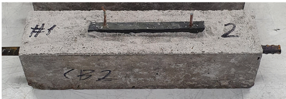
Fig. 1. (a) Schematic representation of the mixing steps of CB-cement paste coatings and concrete substrates. First, concrete is mixed and cast in 40 \text{ mm} \times 40 \text{ mm} \times 160 \text{ mm} moulds. After 3 h, the conductive CB/cement mixture is produced and applied on top of the concrete substrate in 7.5 \text{ mm} \times 3 \text{ mm} \times 80 \text{ mm} silicon moulds. Finally, the (b) composite system is left to cure in water for 28 days.
