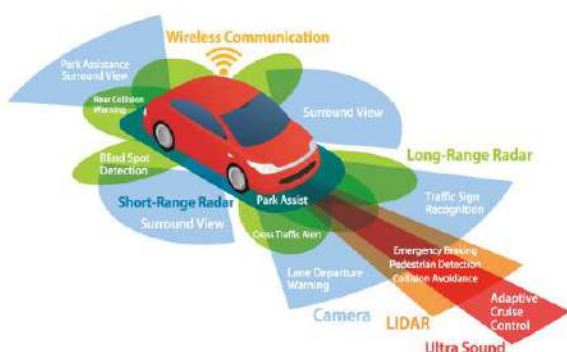
Fig. 7. Smart sensor systems implemented in the autonomous car
