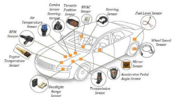
Fig. 6. Implementation of basic smart sensors for obtaining status information
