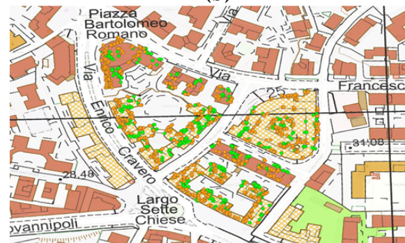
Figure 3. Topographic cumulative distribution of PSs for Area 1 (a) and Area 2 (b). The red dots indicate the cut-off height \delta . The results with removed PSs are shown in (c,d), respectively.
