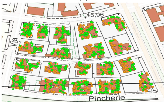
Figure 3. Topographic cumulative distribution of PSs for Area 1 (a) and Area 2 (b). The red dots indicate the cut-off height \delta . The results with removed PSs are shown in (c,d), respectively.
