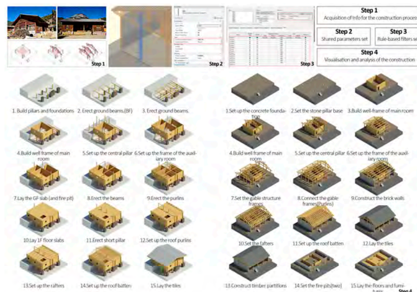
Figure 13. Visualisation and comparison of the construction process of different ethnic minorities (the left is the Nu nationality architectural sample, and the right is the Mosuo nationality architectural sample).
