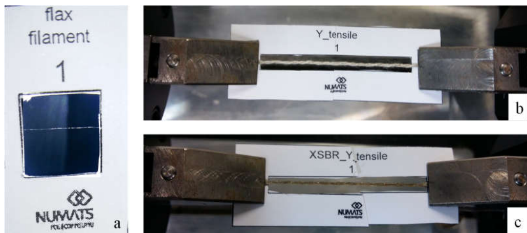
Figure 4. Flax specimens tested in tension: (a) filament; (b) non-impregnated yarn; (c) impregnated yarn.
