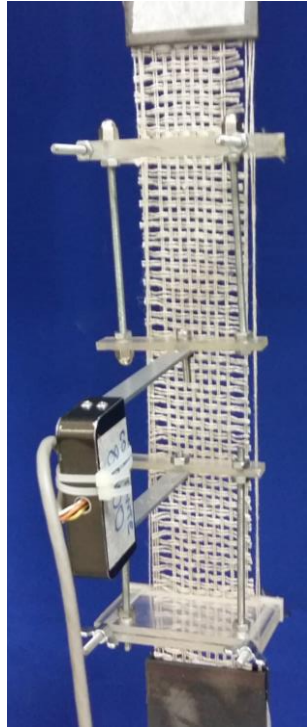
Figure 3. Tensile test set-up for Flax Textile.
