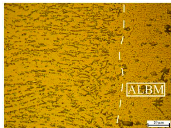
Figure 14. Aluminum nugget in the FREW joint. Reprinted with permission from Ref. [60]. Copyright 2024 Springer Nature.
