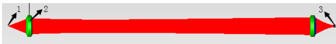
Figure 2. Optical simulation of the two convex lenses, where 1 is the output beam from the paraboloid concentrator, 2 is the convex lens and 3 is the detector.
