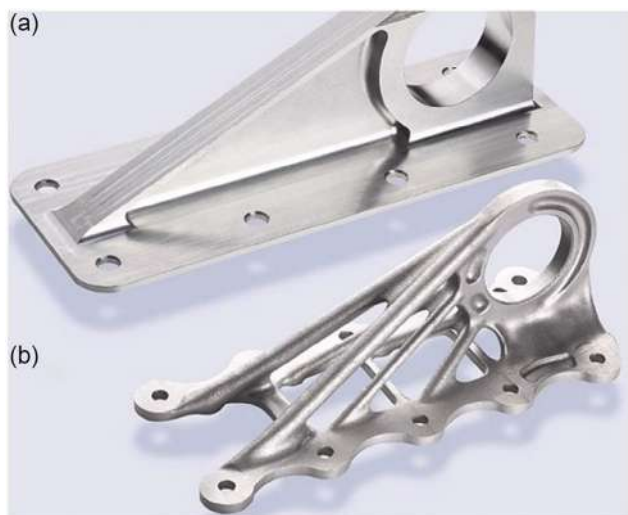
Figure 31. Ti cabin bracket Airbus A350 XWB produced by a) conventional and b) additive manufacturing methods. Reproduced with permission. [178] Copyright 2023, Elsevier.
