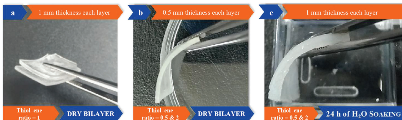
Figure 6. Fluorinated bilayer structures: a) when using stoichiometric polymers no adhesion; b) when combining the off-stoichiometry polymers good adhesion after the photopolymerization reaction c) adhesion is maintained after 24 h of water immersion at RT.
