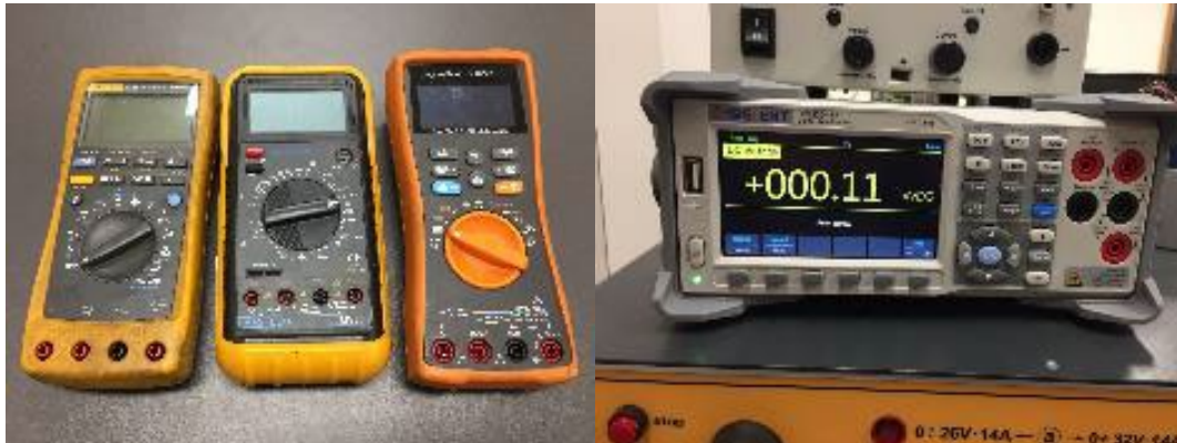
Fig. 3. Handheld and bench multimeters used in the 1 st lab test.
