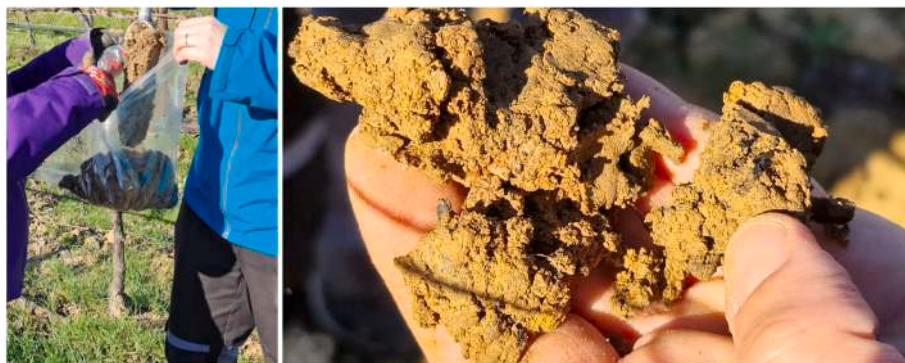
Fig. 5. Auger soil sampling at La Braccasca farm (left) and image of sampled soil with biochar (right).
