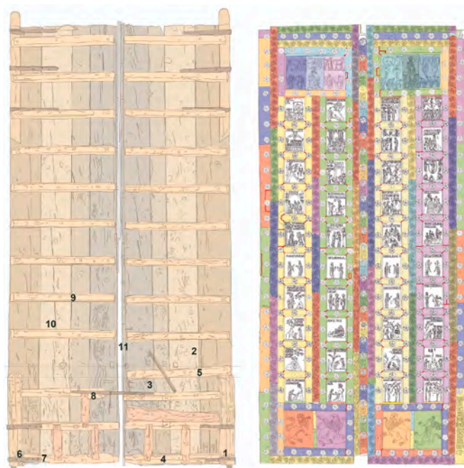
Fig. 3. Monreale. The wooden structure of the door with sampling locations (left) and the different metal elements applied onto it (right). Different colours distinguish the separate elements (© Carlo Usai). (For interpretation of the references to colour in this figure legend, the reader is referred to the Web version of this article.)
