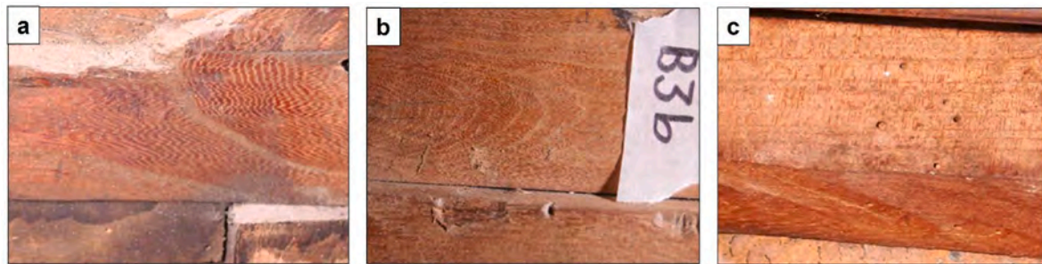
Fig. 21. On the left and in the centre are two sub-transverse surfaces showing the characteristic wavy light lines due to the particular distribution of axial parenchyma. On the right is a radial surface highlighting the parenchyma rays, visible as thin and short dark lines.
