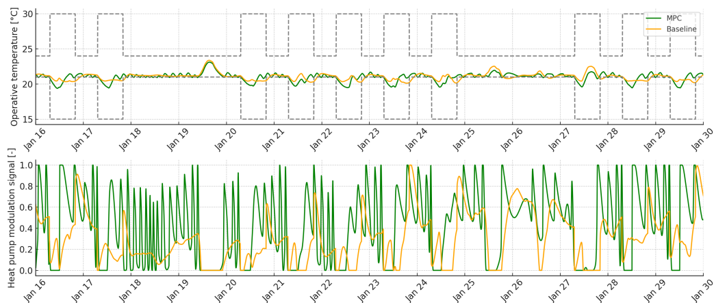
Figure 9. Simulation results for the peak heating period with constant pricing scenario. T_h = 8 h and time step = 5 min.
