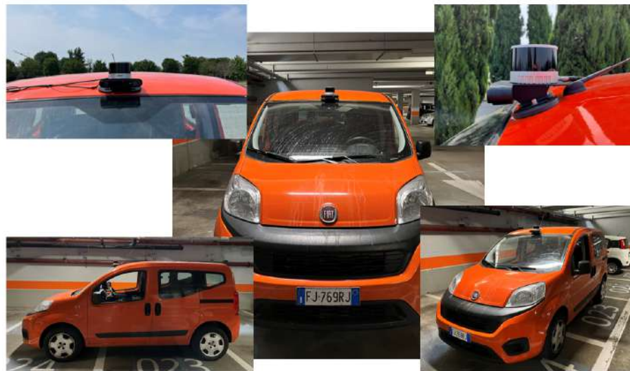
Figure 4. LiDAR and camera mounting position on the vehicle used for on-road data acquisition.
