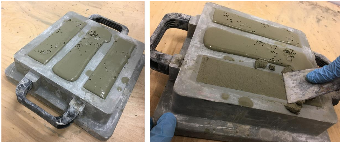
Figure 1. (Left): two-component grout samples cast following Todaro et al. [23]; (right): the sample trimming phase.
