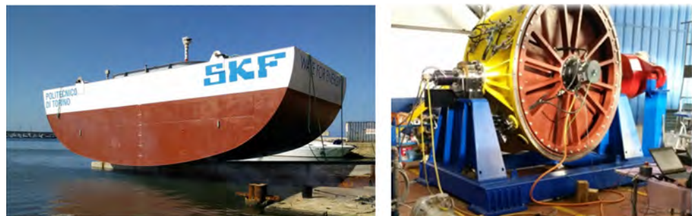
Figure 4. Full-scale ISWEC device during the installation phase (right) and gyroscope mounting process (left). The device was developed by the Politecnico di Torino, Department of Mechanical and Aerospace Engineering.
