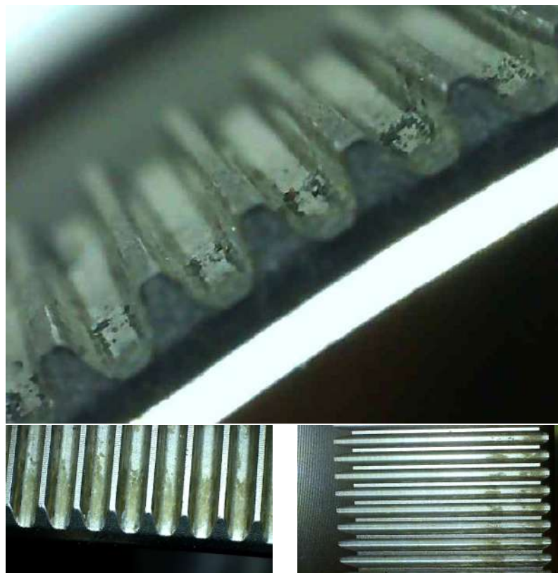
Figure 7. Wear of the flexspline teeth.
