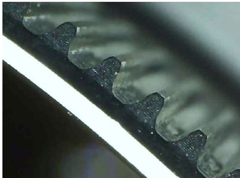
Figure 2. Double-arc profile of the flexspline tooth.
