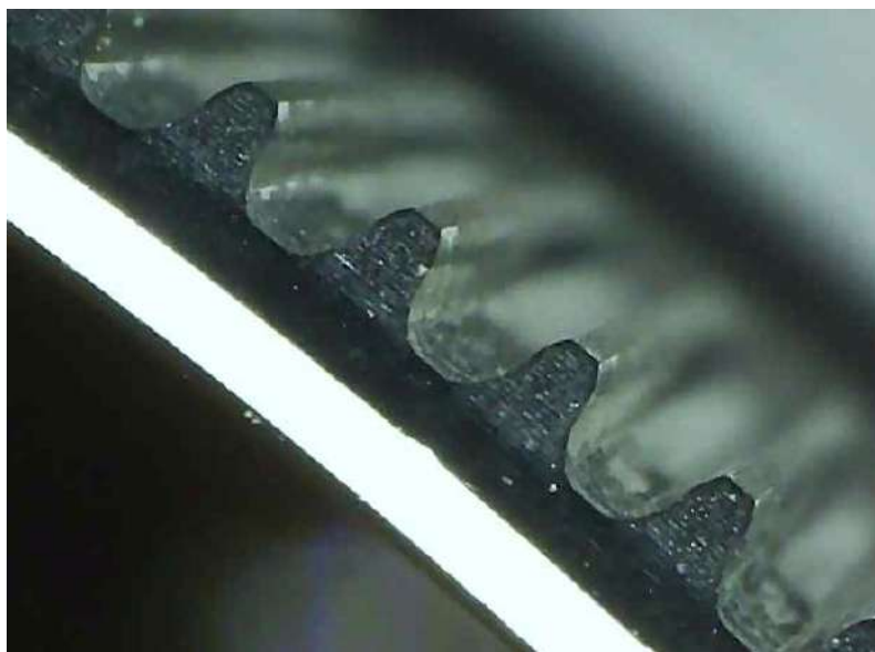
Figure 2. Double-arc profile of the flexspline tooth.
