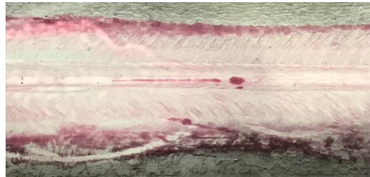
Figure 8. Penetrant liquid inspection result.
