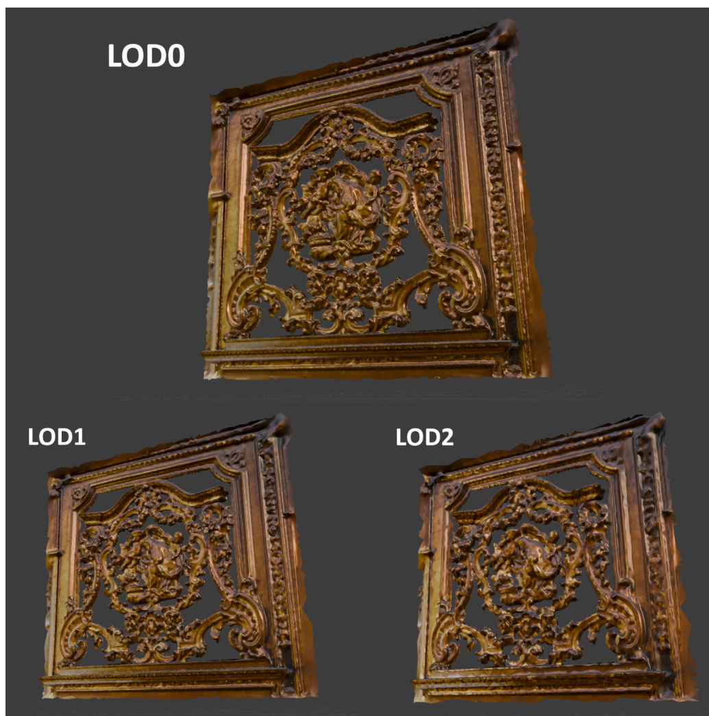
Fig. 6. Representation of the three LODs for one of the reconstructed decorations (the Winter season). For this example, the number of vertices obtained for each LOD was \sim 260k (LOD0), \sim 60k (LOD1), and \sim 15k (LOD2).
