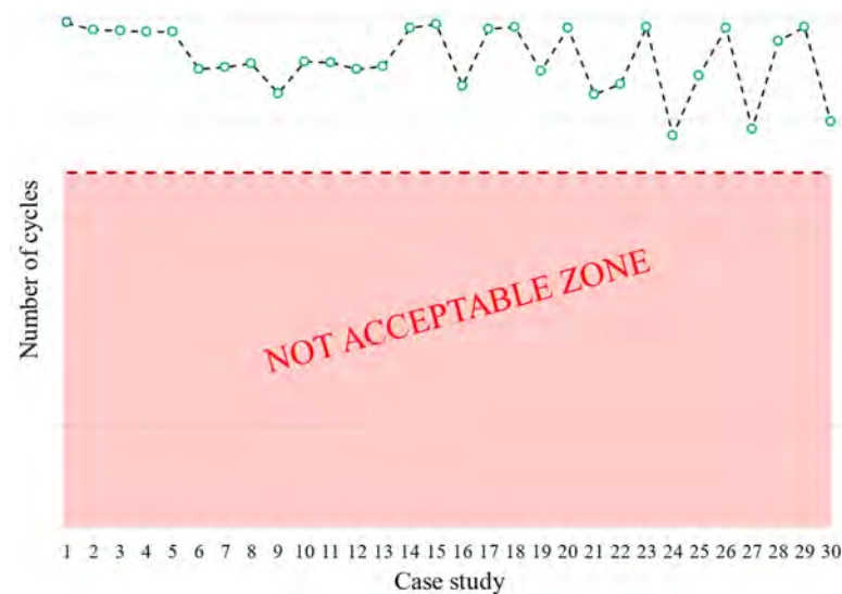
Figure 27. Disc groove: Changes in the number of cycles at crack initiation (LCF) for all of the cases studied compared to the nominal geometry.
