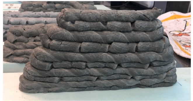
Fig. 3. Result of 2D-printing test conducted on 3DPFC_800.
