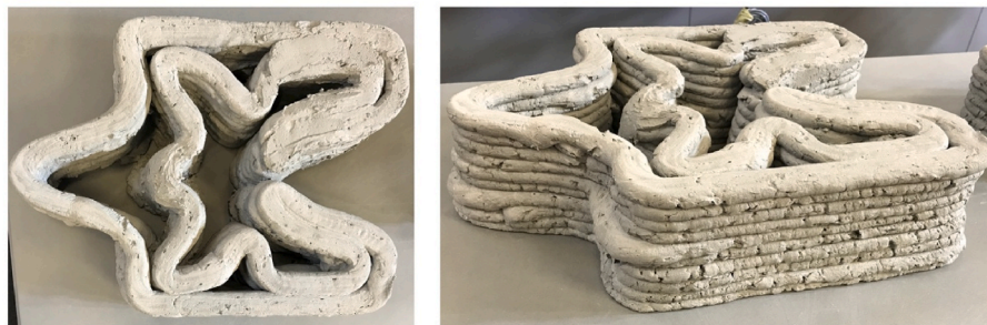
Fig. 12. Representative images of BC.1 obtained using 3DCP.
