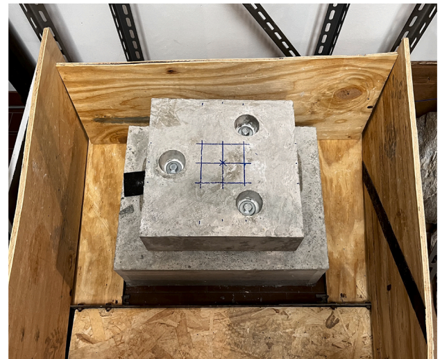
Fig. 1. View of the impacted plate: the center of the 5 × 5 cm grid corresponds to the centroid of the system.
