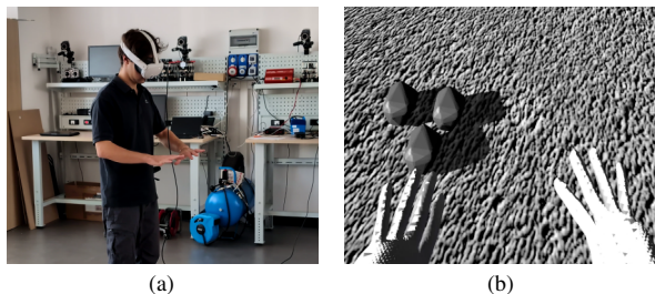
Fig. 3: Mapping of real world movements into simulation: user (a) and rigged avatar (b).
