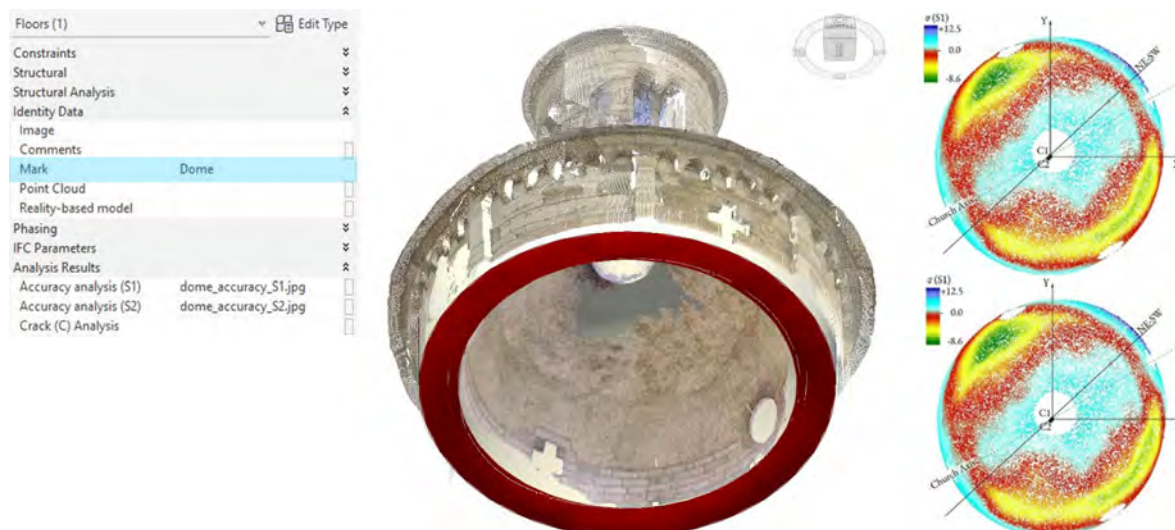
Fig. 7 - Accuracy analysis. Two dome’s scalar fields connected to the dome’s model. (@D. Prati).
