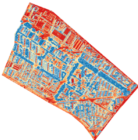
Fig. 8. Solar radiation map, output of r.sun.insoltime .
