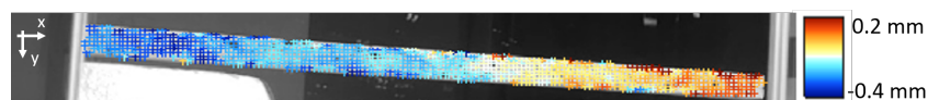
Figure 7: Out-of-plane displacement map of a clamped L-beam excited at its first resonance frequency obtained using the smartphone-based Pseudo 3D-DIC setup.
