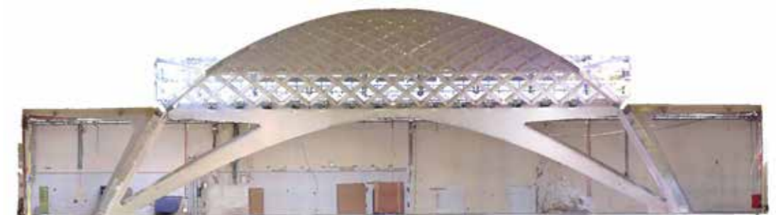
3a 6.5: A projected section of the LiDAR point cloud of Hall C.
