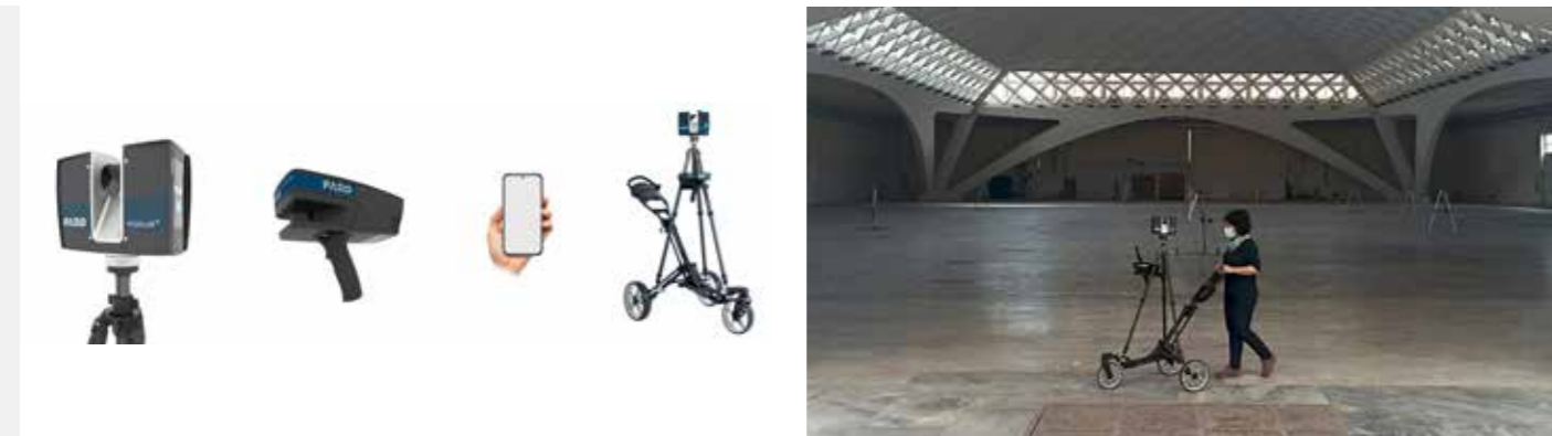
3a 2.2. a, b: The SWIFT system of Faro Technologies: (above) the main components (S series laser scanner, ScanPlan with profilometer that uses SLAM technology to determine the trajectory and the mobile phone that connects the different components); (below) the system is in action in Hall 3 of the Turin Exhibition Center.
