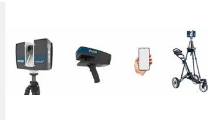
3a 2.2. a, b: The SWIFT system of Faro Technologies: (above) the main components (S series laser scanner, ScanPlan with profilometer that uses SLAM technology to determine the trajectory and the mobile phone that connects the different components); (below) the system is in action in Hall 3 of the Turin Exhibition Center.
