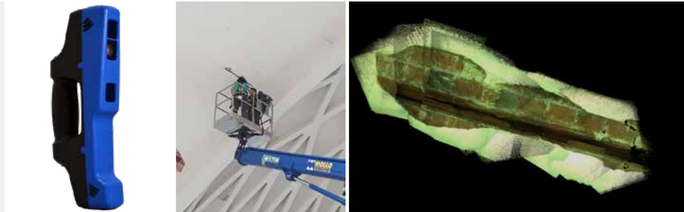
3a 9.8: Stonex F6 SR - The forklift made it possible to reach distances of less than one meter in the great arch that separates the central nave and exedra. A portion of the surface where the investigations operated on the cleaning and removal of plaster due to a pre-existing crack was acquired on a very large scale, as can be seen from the preview shown in the photo.
