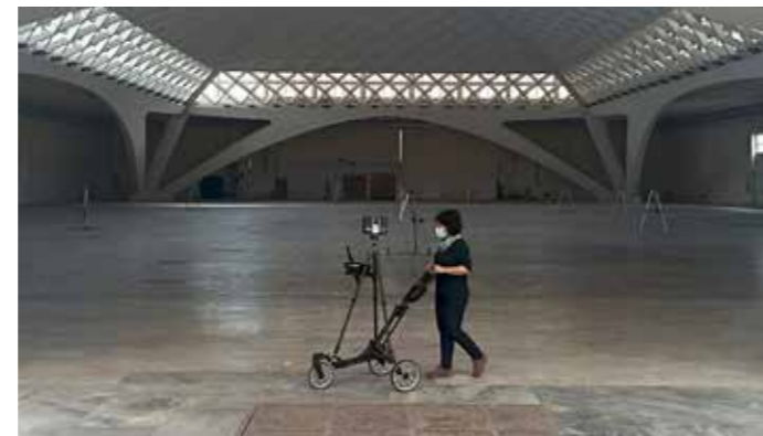
3a 2.2. a, b: The SWIFT system of Faro Technologies: (above) the main components (S series laser scanner, ScanPlan with profilometer that uses SLAM technology to determine the trajectory and the mobile phone that connects the different components); (below) the system is in action in Hall 3 of the Turin Exhibition Center.
