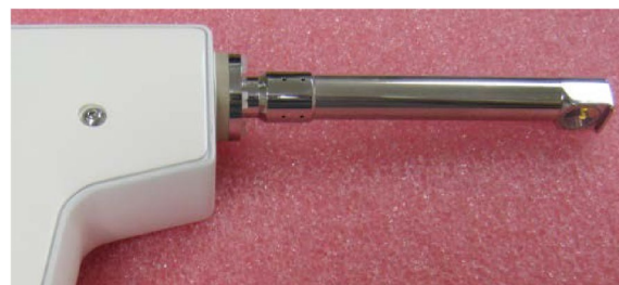
Fig. 1 Prototype of manual probe for intraoral use
