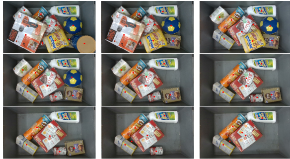
Fig. 2: Picking timeline with SAM for the Easy scenario. An infinity cycle was performed during which the pipeline was shown to empty the box several times. The red dots represent the picking points.
