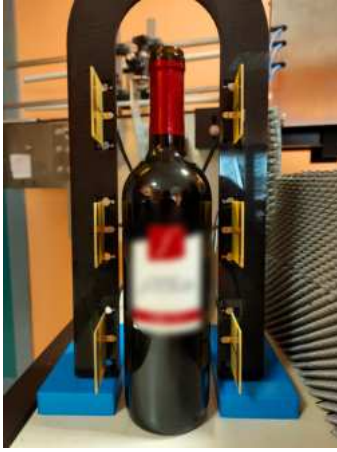
Fig. 1. A commercial glass bottle surrounded by six fabricated prototypes of the PSADEA-optimized antenna to acquire a 6 \times 6 scattering matrix and perform the microwave image reconstruction.
