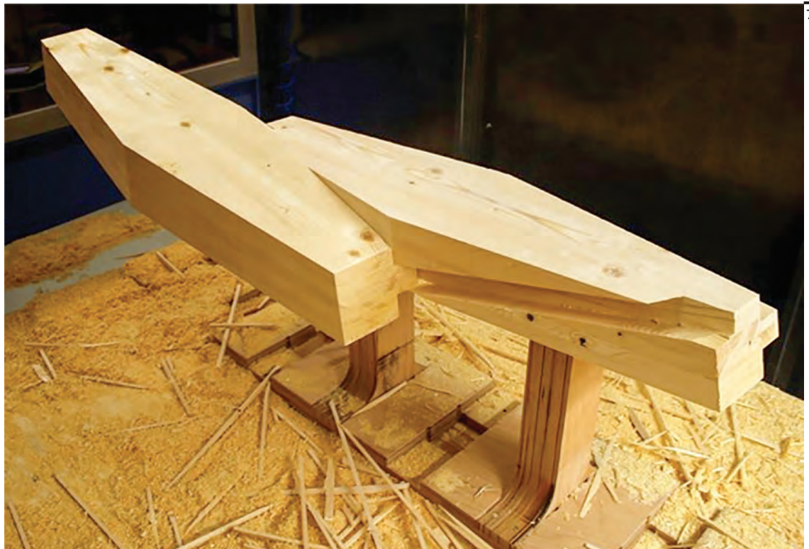
Fig. 7 Hexagon massive timber trunks forming a continuous shell structure by means of lateral wood- wood connections (photo IBOIS).
